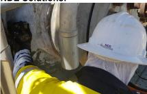
Caption: Available: Advanced NDT Technician scanning a pressure vessel using Phased Array Ultrasonics CLICK HERE
