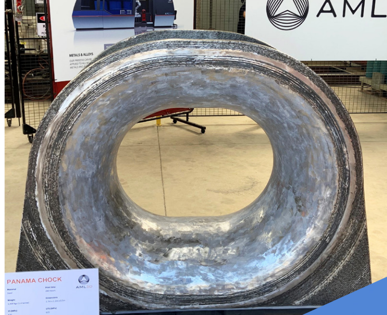
1,400 kg Panama Chock developed for Keppel Corporation in Singapore.
