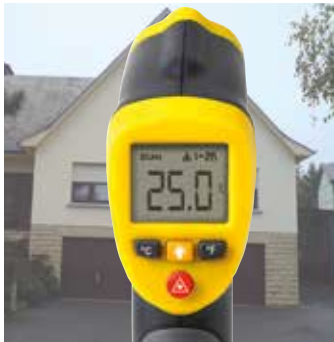
IR thermometer, temperature measurement in one spot
